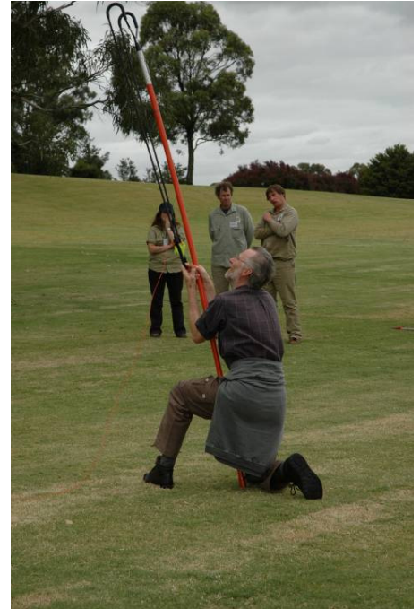
Fig. 5. Pole sling-shot for propelling sandbags over branches
